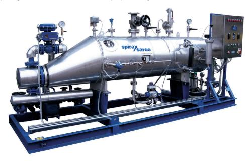
The CSM-K range of high capacity clean steam generators has been designed to provide sterilizer grade clean steam from suitably treated feedwater using plant steam as the heating medium. Units using other fluids on the heating media can be provided to special order.
